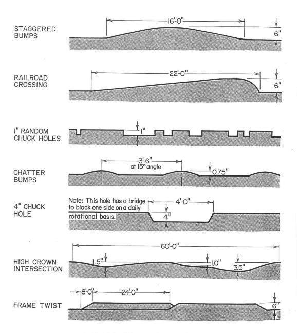
Figure 5.7-2. Side view of stress elements.
